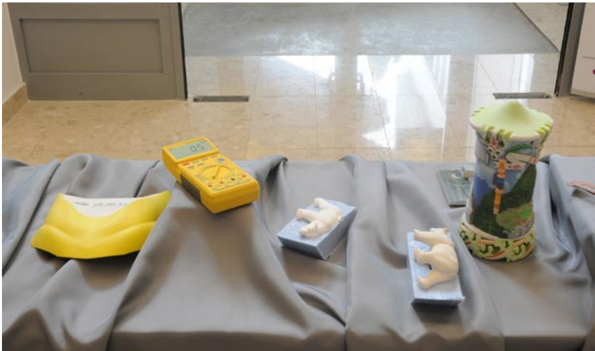
3D samples printed on ZCorp 3D printing machines (rapid prototypers). This class of 3D printing machines use various brands of either thermal or piezo printheads to jet binder (as a glue) instead of ink. The ZCorp uses HP printheads which are thermal printhead technology
