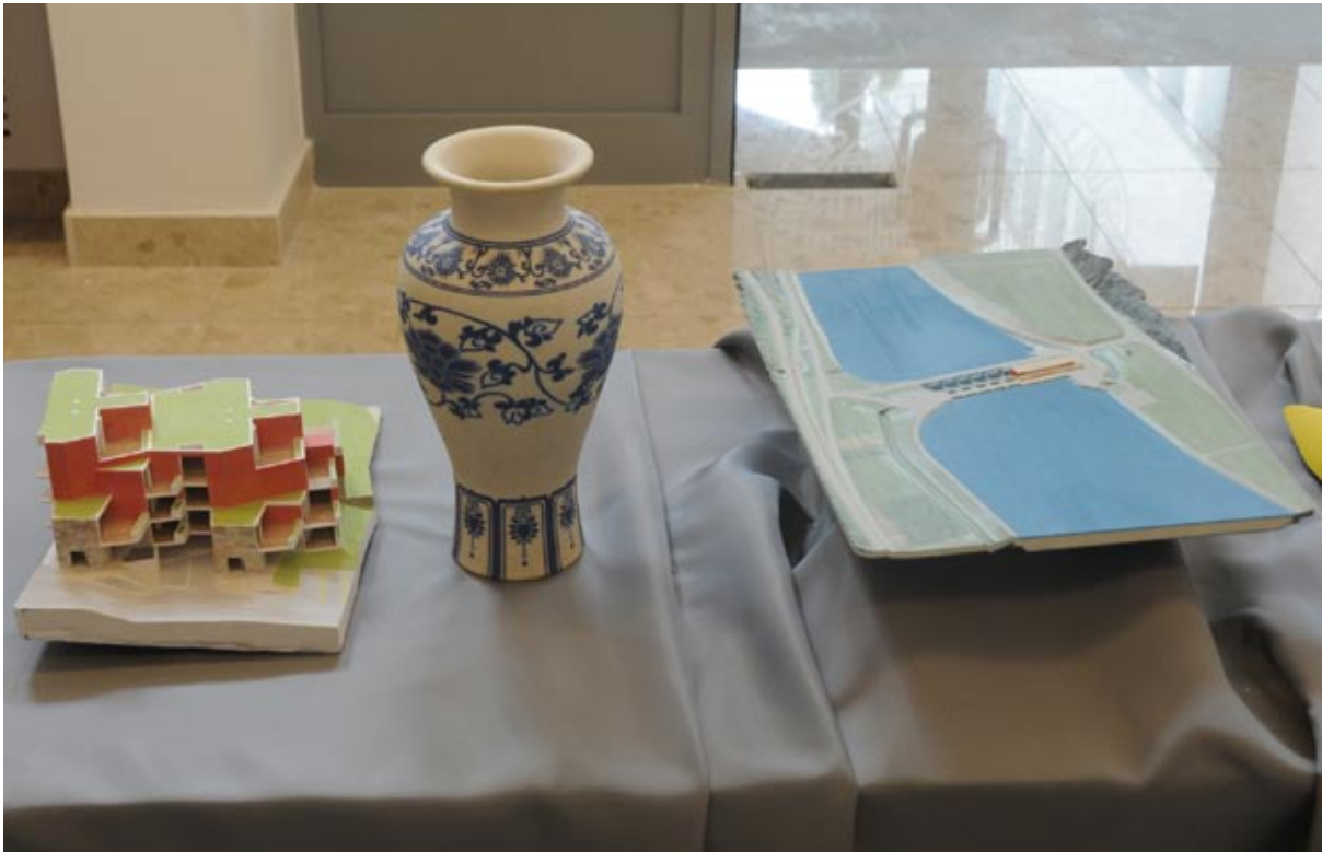
3D samples printed on ZCorp 3D printing machines (rapid prototypers). This class of 3D printing machines use various brands of either thermal or piezo printheads to jet binder (as a glue) instead of ink. The ZCorp uses HP printheads which are thermal printhead technology
