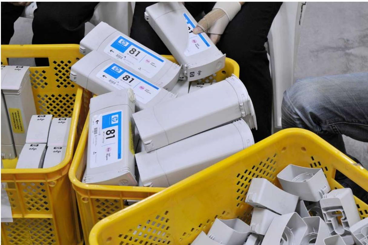
*Here the HP cartridges are being saved from landfill; the original labels are removed. They will be re-chipped and re-branded and re-filled.*
