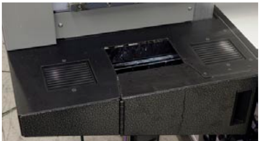
The cleaning area is at left. Here you see the purging tray and the two UV lamp heat sinks.
