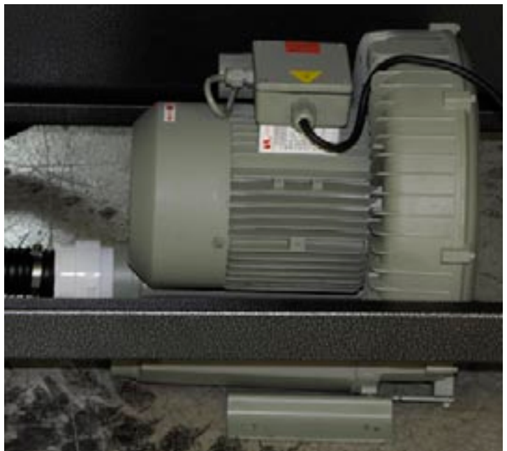
Flat materials are held by the vacuum created by a pump located below the flatbed table.
