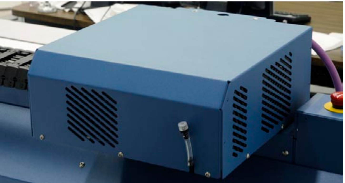
At the back of the carriage there is a secondary fan system.
